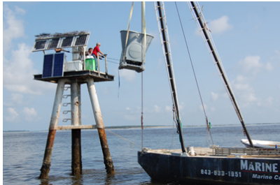
Testing SODAR to measure off-shore wind
