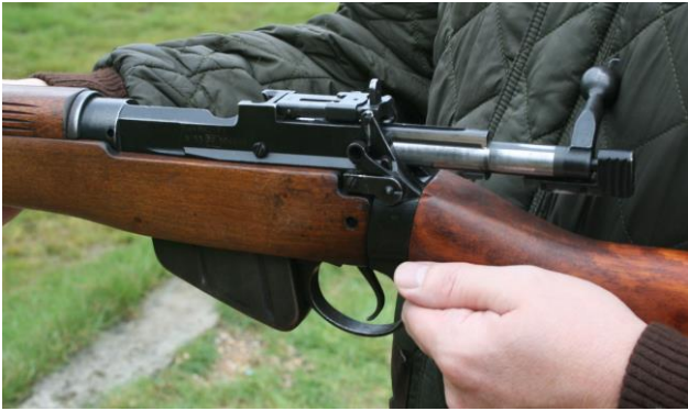
Enfield No 4. Safety catch off, bolt open
