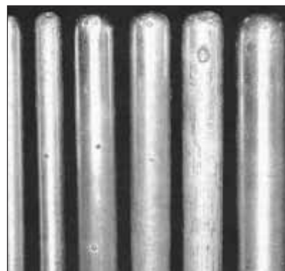
These six blunt aluminum rods used in experiments by Dr. Charles Moore, et. al., show that blunt-tipped rods are better lightning receptors than sharp-tipped rods. In these experiments, done on South Baldy Peak, N.M., 13 blunt-tipped rods were struck by lightning, but none of the nearby sharp-tipped rods took a strike. The two rods on the left were 12.7 mm in diameter, the rod on the right was 25.4 mm in diameter, and the other rods were 19mm in diameter. Source: The Case for Using Blunt-Tipped Lightning Rods as Strike Receptors, C.B. Moore, G.D. Aulich, and William Rison. Journal of Applied Meteorology, Volume 42, page 992.
