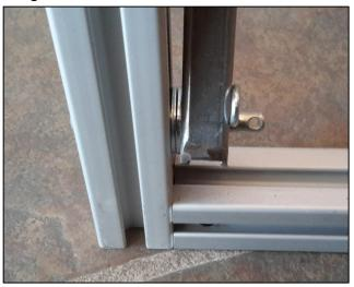
Connect each set of scissors by pinning them together through the holes in the center of each member using a 3.5-inch double threaded rod, 1-inch spacer, and four washers each.
