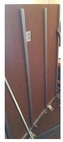
Figure 12: Top Panel Support Structure
