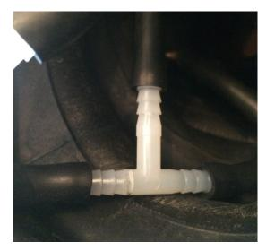
Figure 16: T-Joint connected to vacuum hosing
