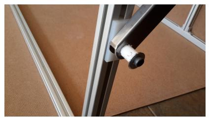
Figure 13: Slider Assembly
