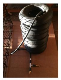
Figure 18: Tire Stack Air Bladder
