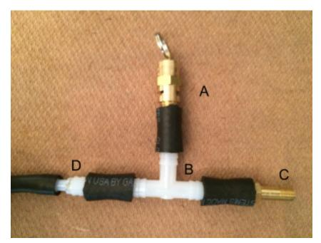
Figure 17: Input, Bleed Connection, and Feed Line Assembly
