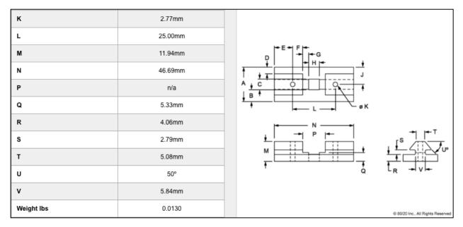
**Figure 8: Critical Slider Geometry**
