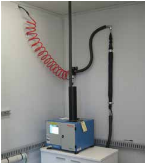
TEOM instrument – used for PM 10
