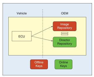
**FIGURE 4** Uptane uses two repositories to provide OEMs with both security and customizability [38], [39].
