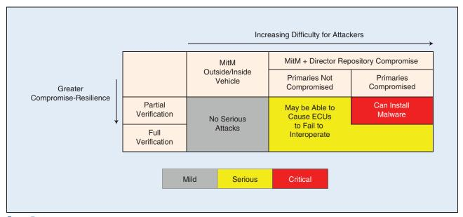
FIGURE 5 A rough security analysis of Uptane, depending on which repositories and ECUs have been compromised [38], [39]. MiTM: Manin-the-Middle.
