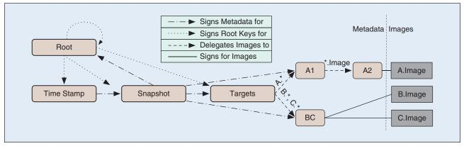
FIGURE 2 The separation of duties between signing metadata roles [38], [39].
