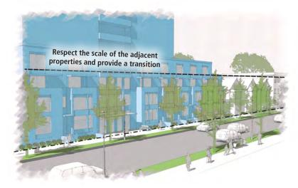
**Diagram 2-7:** A conceptual illustration of the articulation of the base to respect the height and pattern of the abutting existing residential buildings.
