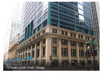
**Figure 1-13:** An example of integrating the preserved heritage elements into a high-rise building. The structure and fenestration of the tower are designed to respect the patterns of the heritage building.
