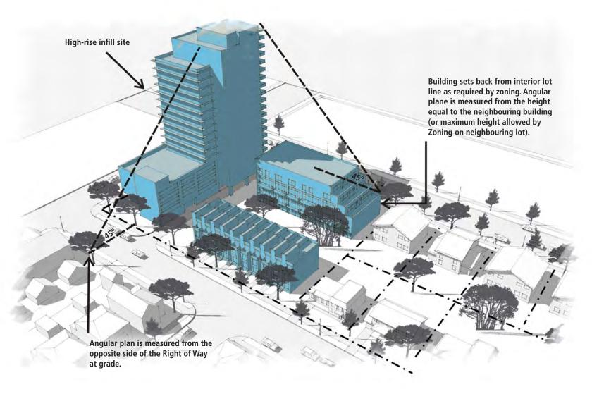
**Diagram 1-6:** A conceptual illustration of the approach to determine the appropriate minimum lot area for a high-rise building, likely applicable in the areas outside of the Central Area and the emerging downtown districts. Two angular planes are applied to define the relationship between the location and maximum height of a high-rise building and the lot dimensions to provide the desirable transition between the high-rise and the adjacent stable low-rise area.
