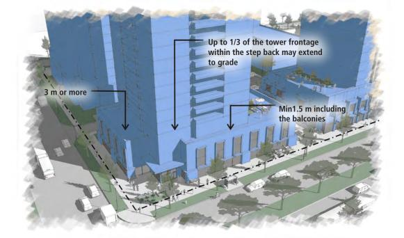
**Diagram 2-11:** A conceptual illustration of tower step backs from the base and the allowance of a portion of the tower to extend to the grade.
