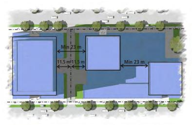
**Diagram 2-9:** A conceptual illustration of the separation distances of towers and the mechanisms to achieve them.
