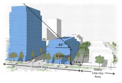
**Diagram 1-4:** A conceptual illustration of a possible application of an angular plane. The rear lot line is the boundary between the stable low-rise area and the growth area. The angular plane is measured from the top of the 4th floor of the building, which is set back 7.5m from the rear lot line. Buildings in the growth area may be under different ownership and subject to a master plan, a CDP or a Secondary Plan.
