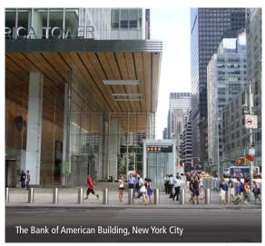
**Figure 3-4:** The pedestrian space below the cantilevered building should be of sufficient height to provide a bright, open, and inviting pedestrian space.
