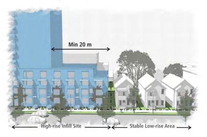
**Diagram 1-5:** A conceptual illustration of the approach to determine the appropriate minimum lot area for a high-rise building, likely applicable in the Central Area and the emerging downtown districts. A minimum tower setback is applied to establish a transition zone between the high-rise tower and the abutting stable low-rise area.
