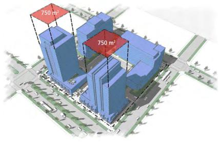
**Diagram 2-8:** A conceptual illustration showing maximum floor plate of 750 m<sup>2</sup> that includes all built areas, including the balconies.
