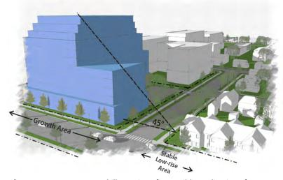
**Diagram 2-5:** A conceptual illustration of a possible application of an angular plane when a bar building is located across the street from a stable low-rise residential area.
