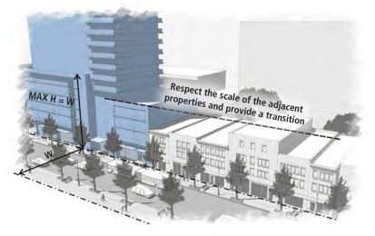
**Diagram 2-6:** A conceptual illustration of the articulation of the base to provide transition in height.
