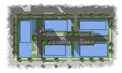
**Diagram 3-2:** A conceptual illustration of a master-planned development where parking is located underground and additional parking, loading and drop-off areas are located in the interior of the development site.
