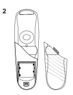
Match the + and – marks on the batteries to the + and – marks in the battery case, then insert the batteries.
