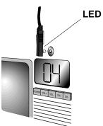
4 Test the *Home Producer*. The Command Center will convert the RF signal from the Home Producer into an IR signal and transmit that signal to your component through the IR signal extension cord.
