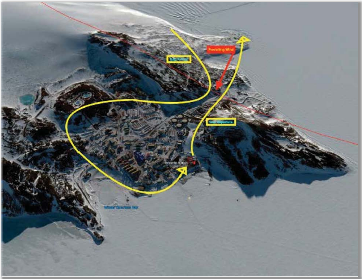
Figure 3.3. shows RW gap arrival and departure routing when prevailing wind is from the Scott Base.
