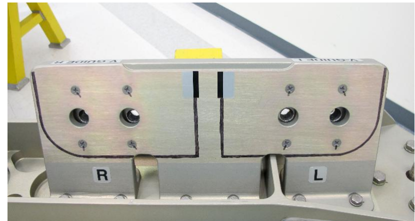
Sharpie Alignment Marks on RGB
