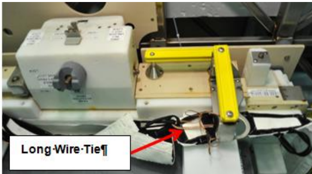
Tie down of flaps near Primary Bolt
