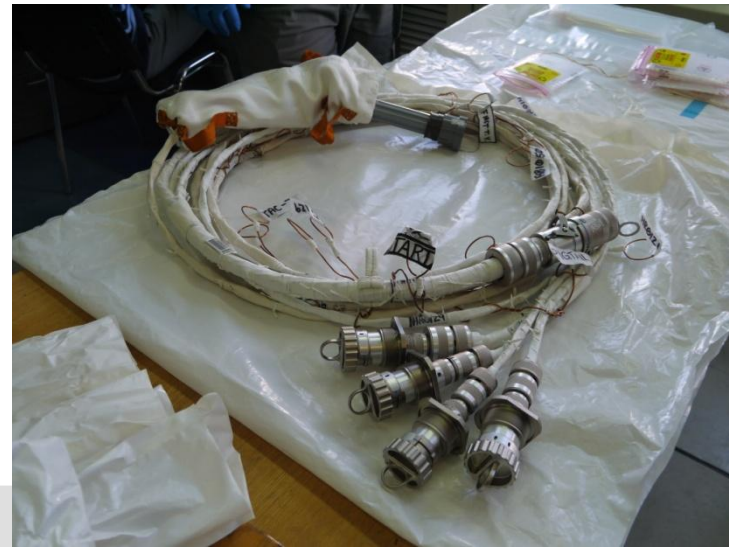
Ground photo of cable post RS connector integration.
