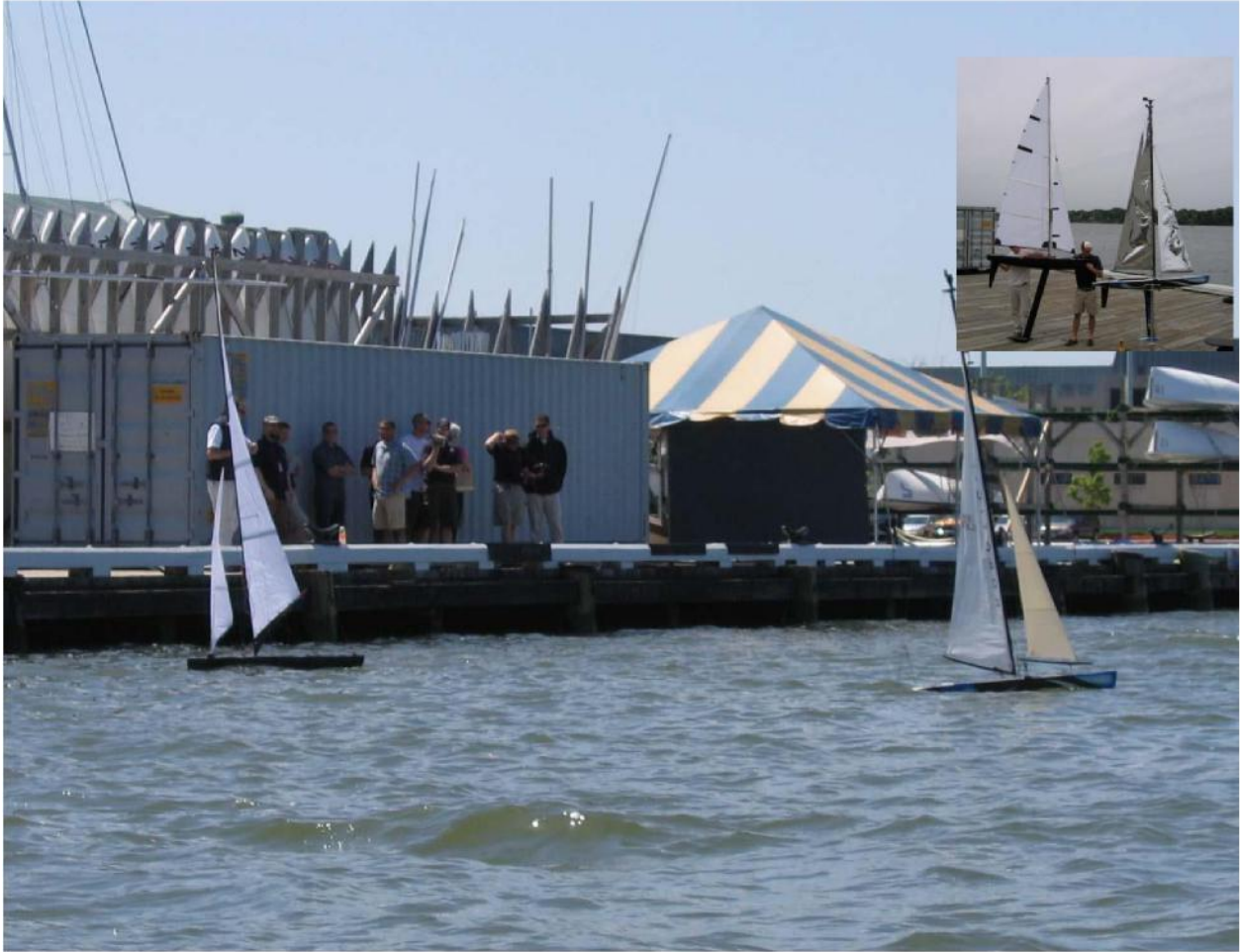
Event of the Future? “Robotic” sailboats (SailBots) competing at the United States Naval Academy. College teams design, build and race these boats at SailBot competitions. The boats use onboard computers, instrumentation, GPS and some luck to steer and trim sails around different courses. The insert (upper right) depicts the relative size of these boats. Even with advances in technology, competitors depend on US Sailing Judges to adjudicate issues and incidents during the event.
