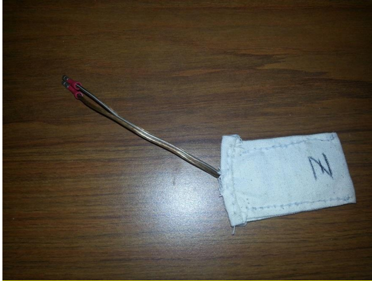
Figure 2.8: Sensor in Canvas, Leads Wired for Harness Attachment
