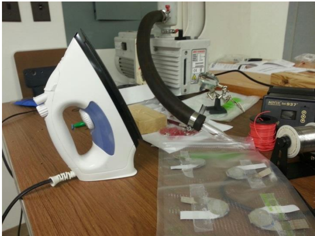
Figure 2.6: Vacuum Seal Bag, Vacuum Pump, and Iron
