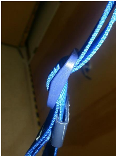
Figure 4.1: Harness 1 Thigh Strap Adjustment
