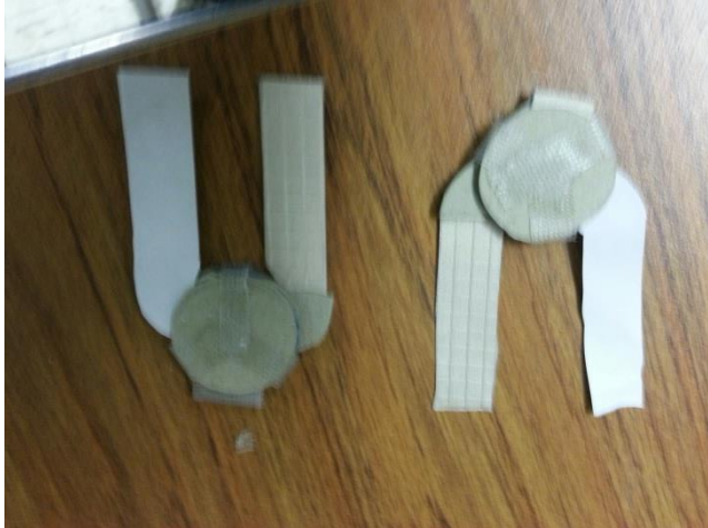
Figure 2.4: Assembled Sensors Before Vacuum Seals
