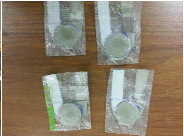
Figure 2.7: Sealed and Cut Out Sensors
