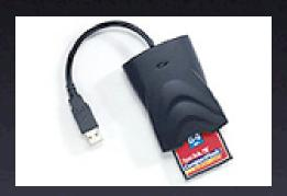
Recognized & mounted by operating system as an external drive
