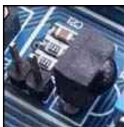
Infrared remote-control receiver – to practice infrared remote-
