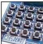
4*4 Matrix keyboard – to test password lock and other items.
