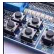
5-way independent key-press—for easy various key-press input experiments.
