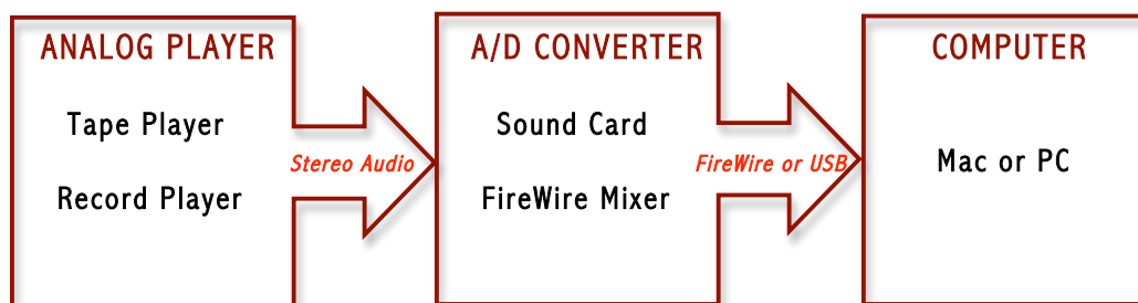
Figure 1. Connection of Audio Equipment
