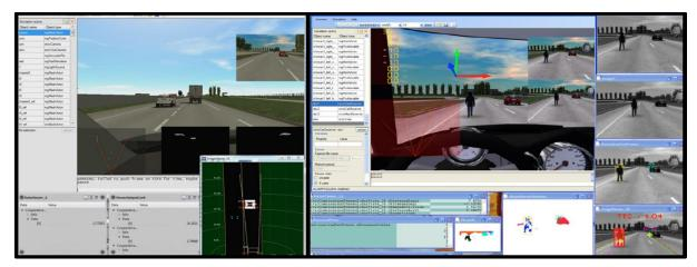
Figure 4: Examples of Pro-SiVIC use for virtual sensors and ADAS simulation
