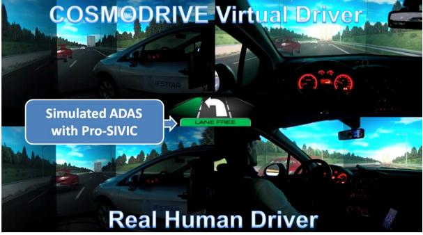
Figure 7: comparative evaluation of ADAS (with virtual vs real drivers) on the V-HCD platform, interfaced with IFSTTAR driving simulator
