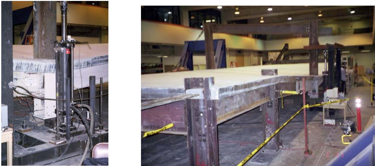
Figure 3.1. Actuator Used to Apply Additional Gravity Load to Floor
