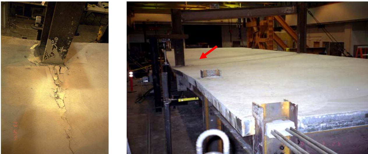
Figure 6.2. Appearance of Slab at the End of 19-Inch Drop Test
