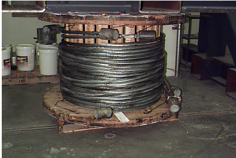
Figure 2.13. Steel Cables As Delivered to the Laboratory
