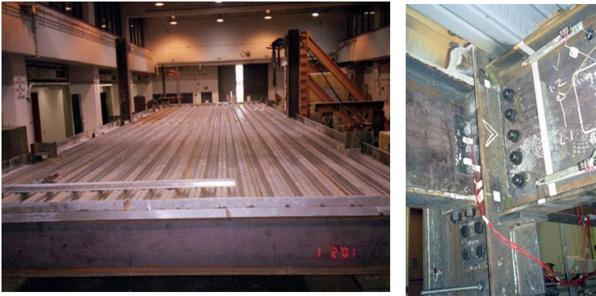
Figure 2.12. Steel Deck (left) and Typical Bolted Connection
