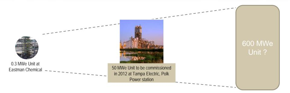
RTI and DOE/NETL's Computational and Basic Sciences Group are using CFD modeling to assist in the design of HTPD for 50 MWe Prototype Unit
