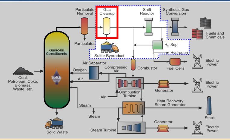
**R&D objective:** Platform of warm syngas cleaning technologies providing improved efficiency, environmental performance, and cost
