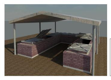
Figure 3: Design for a 1MT capacity ZECC (Kitinoja, 2010) Digital illustration credit: Amity University, Uttar Pradesh, India
