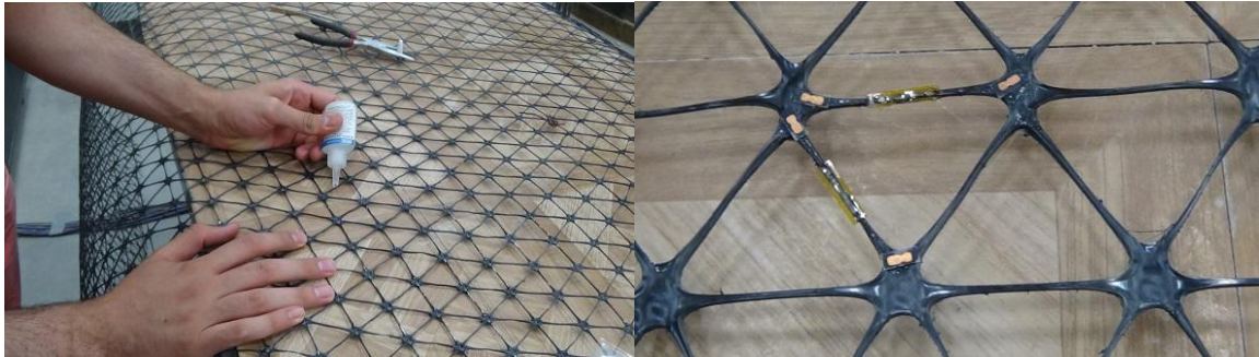
(a) (b) Figure 3.6: Foil strain gauge installation
