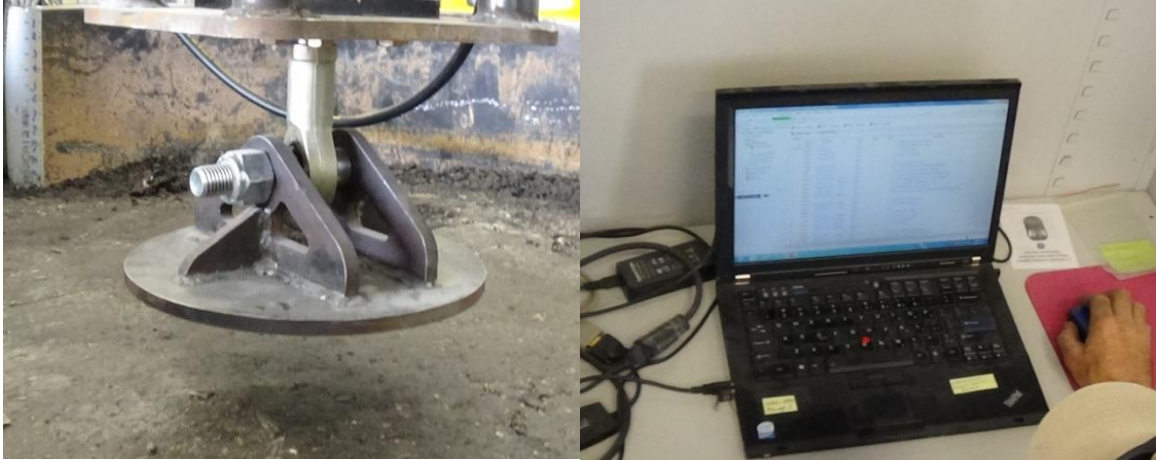
(a) (b) Figure 3.10: Dynamic loading system
