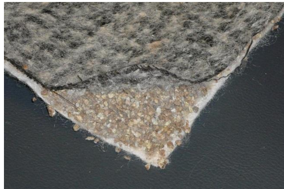
Figure 2.7: Geosynthetic clay liner (Hillier, 2008)
