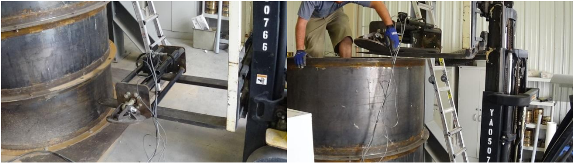
Figure 3.15: Loading plate system installation
