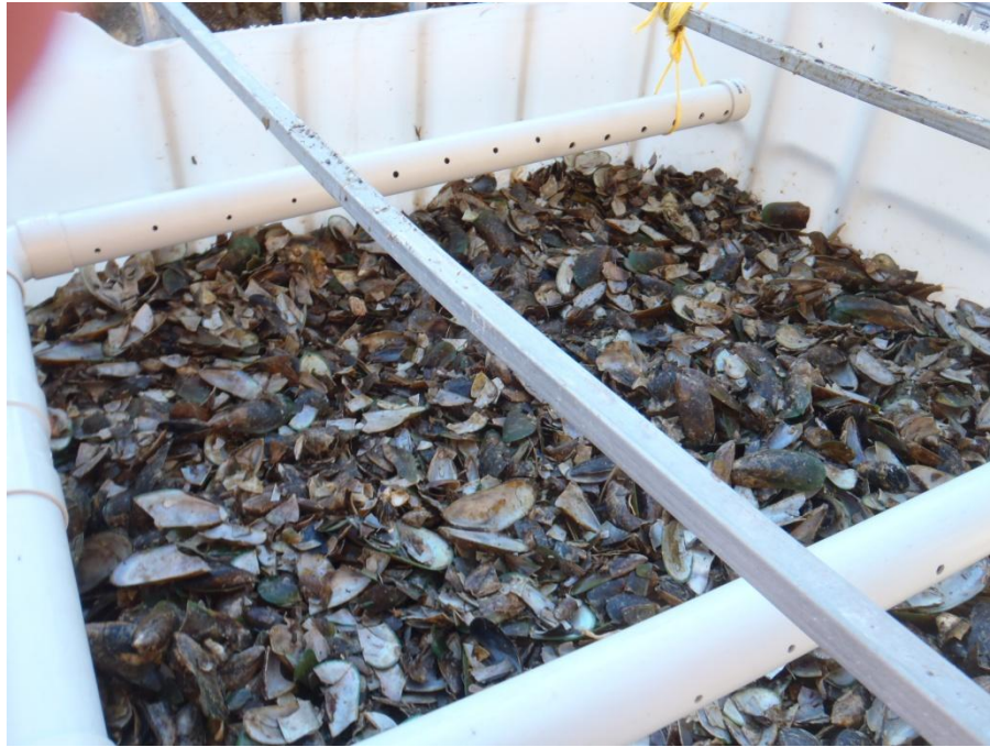
Figure 1. Mussel shells in completed mussel shell reactor prior to filling with water.
