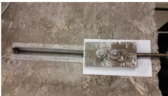
Figure 10 – Test series 15 – Steel failure longitudinal shear
