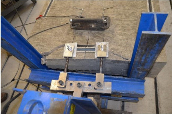
Figure 7 – Test series 10 – Concrete failure shear load
