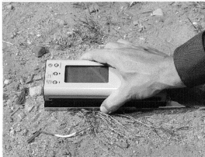
Figure 3. In-situ testing of soil by placing XRF directly onto the ground. This type of testing is generally screening level data quality.
