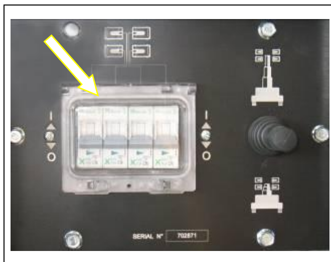
Figure 6.4 – Light control switches
