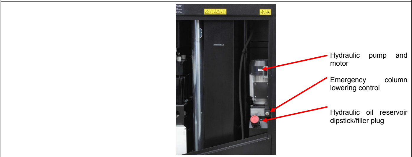
Figure 2.2 – location of the control box, control panel and hydraulic unit
