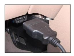
**OBDII Connection** on cable connects to the vehicle if required for relearn
