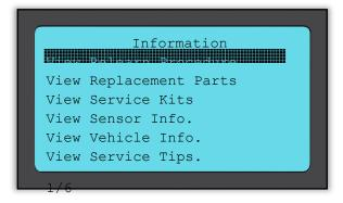
Follow the shown steps on the screen to properly relearn new sensor IDs to the vehicle.
