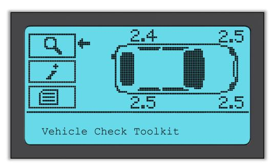
If you go back to the Vehicle Check screen, you can use the arrow keys to move the arrow to the Vehicle Check Toolkit and press the Enter button.
