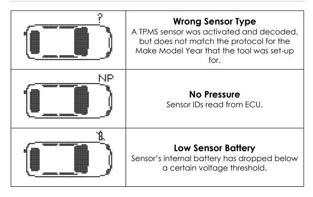
**Note** that if a faulty TPM sensor has been replaced, some method of relearn procedure will need to be followed, as explained later in this manual.
