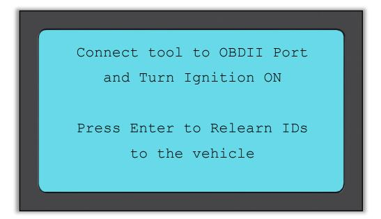
Plug in the OBD II cable and then turn only the ignition on, you should not need to start the engine. If you cannot find the OBD location right away, please use the "View Vehicle Information" menu and select "View Vehicle Info." the tool displays now where the OBD is positioned.
