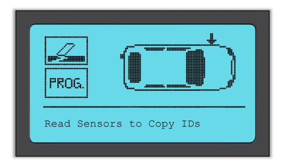
Copying a sensor requires the read of the old sensor to program the same ID on the replacement sensor to avoid the relearning process.
