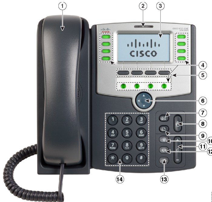
Figure 1 SPA509G Phone Components
