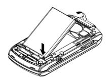
• Replace the cover, making sure all the locking tabs of the cover are seated with no gaps.
