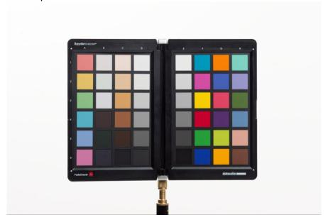
Use a tripod to support the camera whenever possible. Make sure the camera is directly in front of the target. The central axis of the lens should be in line with the center of the SpyderCHECKR. Mount the SpyderCHECKR as suggested above.
