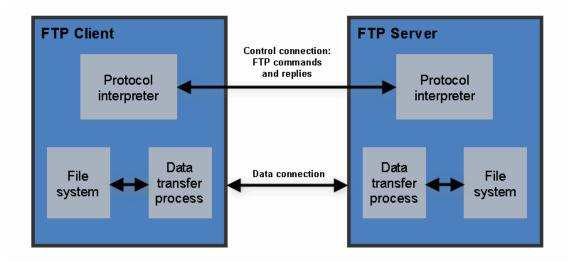
Both the client and the server have a protocol interpreter. The protocol interpreters receive commands or replies, send commands or replies, and govern the data connection. The server's protocol interpreter *listens* for a connection from a client's protocol interpreter.
