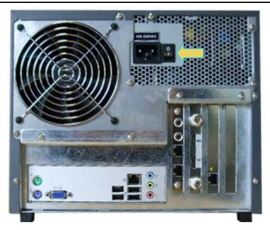
**Note**: The power switch in the front is used when you are turning off the 980 Protocol Analyzer for a short period of time. For extended off periods, it is best to power down the 980 Protocol Analyzer by first using the power button on the front and then the rocker switch on the back.
