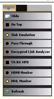
4. Set the TX-RX HPD to replicate the hot plug signal from the TX side (an attached sink device) on the RX side (like a hot plug repeater).
