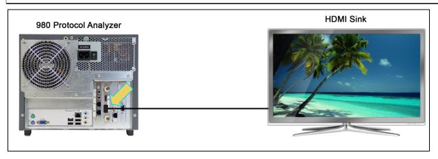
1. Connect your HDMI sink device under test to the HDMI Tx connector (the bottom most HDMI connector shown in the figure above) on the 980 Protocol Analyzer. Use a high speed HDMI cable.
