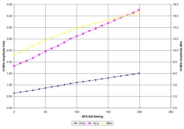
Figure 17 Setting NFS-220 10 MHz output level
