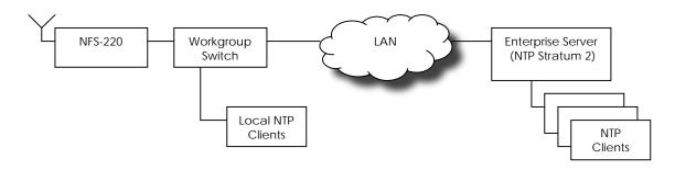
Figure 1 Typical NFS-220 NTP Server Network Connection
