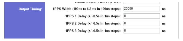
Figure 18 Output Timing Settings
