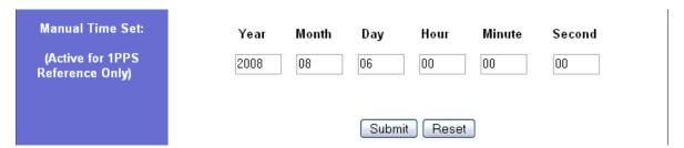
Figure 15 Manual Setting of Time in NFS-220
