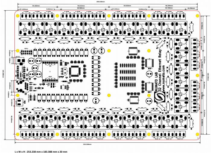
Mechanical Hole Diameter : 4.0 mm
