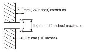
Note: Example above for mounting SBV5220 on a wood surface.
