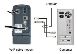
**USB:** Be sure the SURFboard VoIP Cable Modem CD-ROM is inserted in your CD-ROM drive. Perform the appropriate procedure for Setting Up a USB Driver for your Windows version. Connect the USB cable to the USB port on the VoIP cable modem. Connect the other end to the USB port on your PC.
