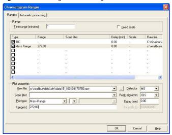
With only the m/z 272 ion shown, it is apparent that the OFN is around a retention time of 3.45 minutes.
