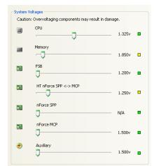
you are no longer in the safe range. If the indicator square is red, you are possible overvoltaging the component and could be causing damage.
