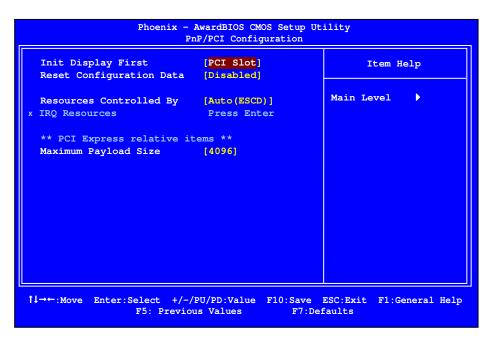
Figure 15. PnP/PCI Configuration Menu
