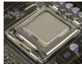
Align notches with notches on the CPU
