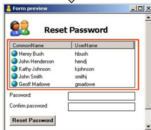
Figure 6 – Reset password delegation project. The result of the LDAP query is displayed in the LDAP table (shown here with a red marquee)
