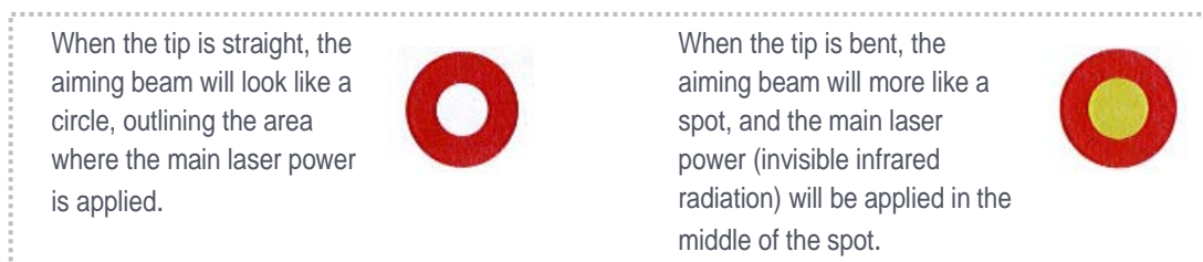
Figure 4-3: Aiming beam pattern.
