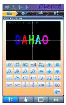
There are 4 rows of operation keys in the interface, the first two rows are the file and view functions keys, the third row are keys for adjusting letter arrangement, and the fourth row are keys for adjusting letter string. In the middle of the interface is the letter pattern display area.
