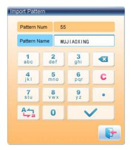
The system provides the minimum available pattern number as the default value. User can use the keypad below to change the number.
