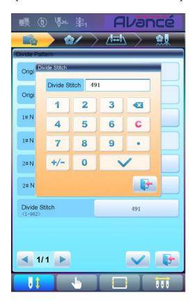
7. Press to divide the pattern into two new patterns and return to pattern operation selection interface. Press to quit the dividing operation and return to pattern operation selection interface.
