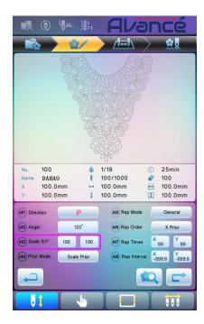
System will display independently the modification windows for X Scale and Y Scale for users to set respectively.
