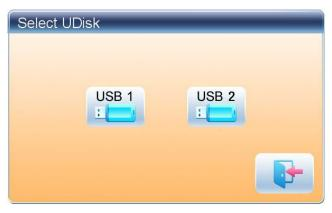
In this window all the storage devices will be displayed. Their information includes the icon, words and numbers. The icon is the device type. Icon indicates U disk. The words are the label of the U disk (if the U disk has no label, the default letter will be used), and the number refers to the U disk's digital symbol.
