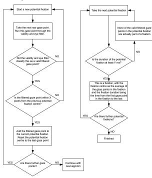
Figure 28: The fixation filter algorithm
