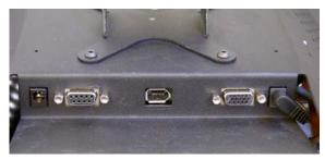
Figure 4: On the back side of the Tobii ET 17 four cables are connected, from left to right, power, serial, Fire wire and monitor cables
