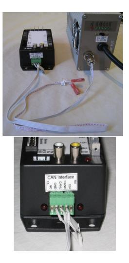
If both the CAN communication and the digital inputs are connected CAN communications will take priority over the digital input for charge control. CAN communications requires the optional CAN board be installed on the BMS CPU.
