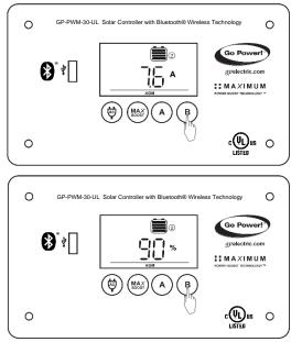
Push the **B Button** to show the PV charging current for battery 2. The GP-PWM-30-UL will begin to limit the current as the battery 2 reaches a full charge.
