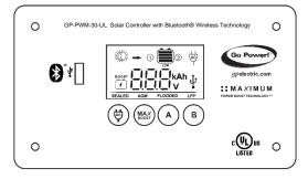
If the GP-PWM-30-UL experiences a battery over voltage (>15.5 VDC) on battery bank 1, the controller will stop operating, and the display will begin to flash with all icons. The controller will resume operating when the voltage drops to a normal level <15.5 VDC.
