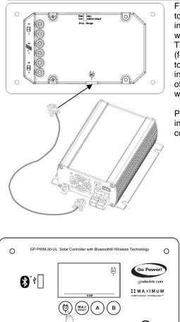
First, connect the inverter directly to the battery (follow the installation instructions included with the inverter). Then, connect the modular cable (found in the inverter remote box) to the remote terminal of the inverter and to the remote terminal of the GP-PWM-30-UL (marked with an **AC Plug symbol**).
