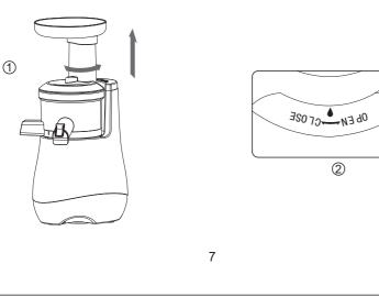
3.Hold the juicer outlet on the squeezing cup shake it lightly and take it out  $(\mbox{see the figure } \ensuremath{\Im})$  .
