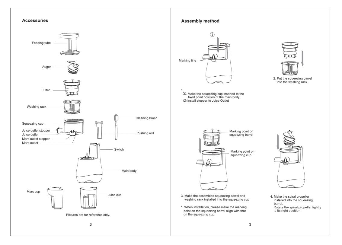
Marking point on squeezing body cover Marking point on squeezing cup
