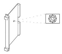
The hex switch is yellow with the scale from 0 to F around it and it is located in the center of the upper third of the modules. The hex switch can be set to the desired value using an appropriate tool. To avoid conflicts during initialization, the addresses must be unique.
