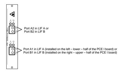
Figure A–11: Front panel of the STM-1 (Tx/Rx) optical line interface
