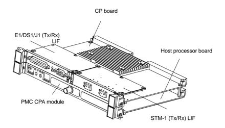
Figure A-9: ATM PCE I board combination
