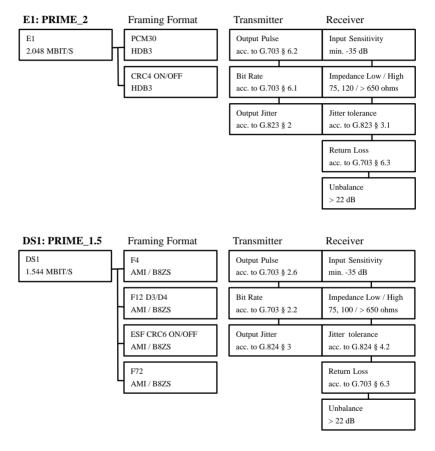
The interfaces of the E1 and DS1 modules implement the physical and electrical connections to the PCM section. For simulation, the sockets feature a transmitter and receiver each for PCM signals. For monitoring, two receivers of the adjacent simulations each are used and combined on a socket.
