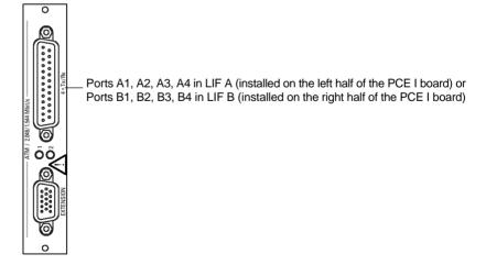
Figure A-13: Front panel of the E1/DS1/J1 (Tx/Rx) line interface
