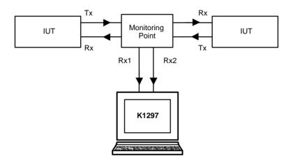
Protected monitoring points can send either E1 data (75 Ohms asymmetrical or 120 Ohms symmetrical), DS1 data (100 Ohms symmetrical), or J1 data (110 Ohms symmetrical). Depending on this type of data, you must select the required cable.
