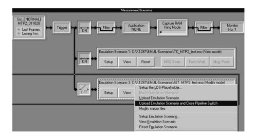
Figure 6: Context menu with Upload Emulation Scenario and Close Pipeline Switch
