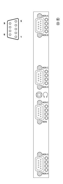
Figure A-6: E1/DS1 monitoring board (PRIMO)
