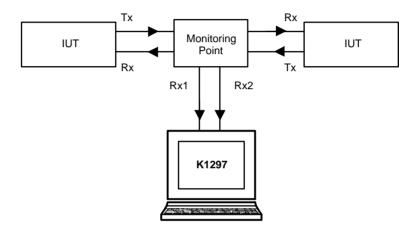
Monitoring points transmit optical signals either in singlemode signals or in multimode fashion. Depending on the transmission mode, you must select the required cable.
