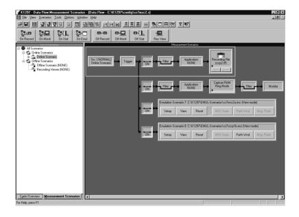
The left pane, List of Scenarios, displays the available measurement tasks (scenarios) as well as the measurement tasks currently configured and the outline sources. On the right, the Measurement Scenarios pane displays the pipelines assigned to the measurement tasks.
