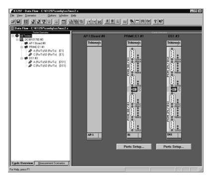
The left pane, <code>Tester Overview</code>, displays the interface modules, ports and the line configurations currently set. The right pane, <code>Cards Overview</code>, shows the individual sockets on the cards including module designation.
