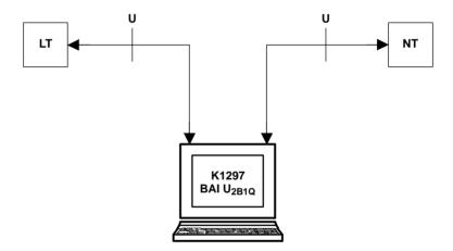
The clock pulses are derived from the LT and transferred to the NT.
