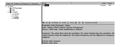
Figure 7: Starting the emulation using the Connect action
