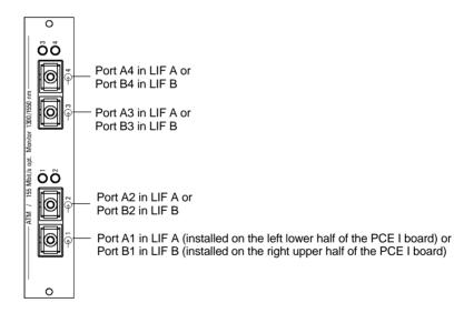
Figure A-12: Front panel of the STM-1 (Rx/Rx) optical line interface
