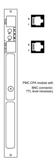
Figure A-10: Host Processor Board
