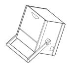
2. Pull the dark grey handle above the logo and lift the keyboard from the device.
