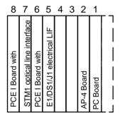
Figure F-1: Board combination (example)
