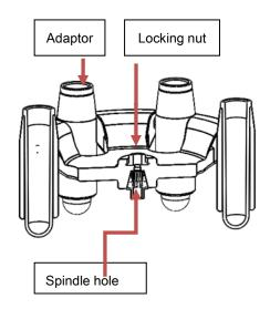
Figure 12-1 Rotor structure
