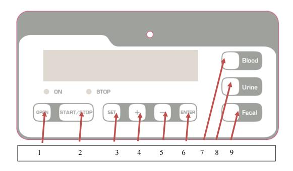
Figure 7.1 Layout of operation panel
