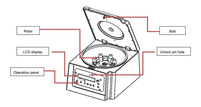
Figure 6.1 Front view of the centrifuge
