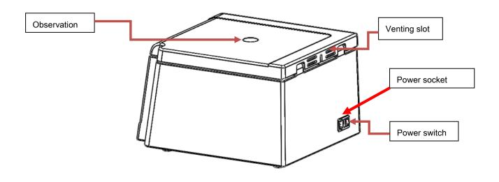
Figure 6.2 Rear view of centrifuge
