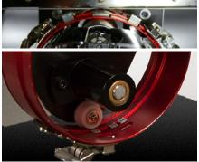
4. Place a business card of medium to heavy stock (or equivalent) between the needle plate and the driver ring. This will act as a spacer. The ring should just rest on the card.
