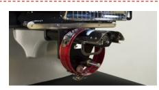
8. Move the driver and carriage back until the cap support wing assembly fully covers the needle plate.
