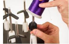
3. Releasing the clover will cause it to expand inside the cone core and stabilize the thread cone.
