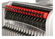
4. Pull the thread from the hole and place it under the pinch roller. Bring the thread down through the upper thread guide.
