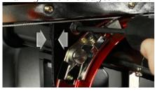
6. Tighten the opposite screw securing the bearing mounting block.
