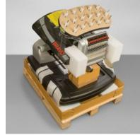
4. Cut the packing/holding straps securing the machine to the box/pallet. Remove any additional loose packaging, boxes, and foam spacers.
