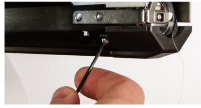
3. Remove the needle plate by removing the two allen screws that secure it.
