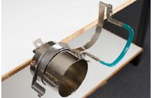
3. Place an appropriate backing over the gauge and the teeth of the cap frame. Make sure that the backing is long enough to support the full embroidery area. It may be easiest to use backing long enough to reach the teeth on each side of the cap frame.
