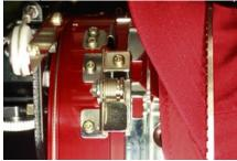
4. With the frame aligned, press the frame toward the driver until the three (3) spring loaded locking clamps snap into place. It may be helpful to grasp the back of the driver and close your grip to
