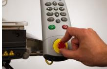
4. <u>Power up the machine with the power switch</u>.
