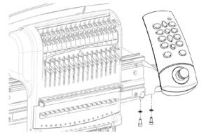
Using the two screws and two lock washers that came with the user interface assembly, attach the interface as shown in the image using a 4mm hex wrench.
