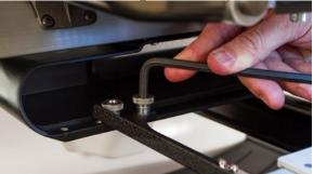
If the hoop brackets shift forward and back, the spring clip may need to be adjusted. See the information below.
