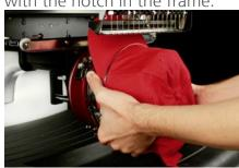
3. This also aligns the rectangular holes along the edge of the frame with the spring loaded locking clamps on the driver.
