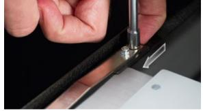
3. Hold the block in place while tightening the nuts.
