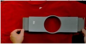
8. Press the hoop down and into place. Take care to press on the ring rather than on the arms. Pressing on the arms can bend the hoop out of shape or break it.
