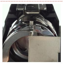
The retaining finger gauge should slide between the hook support an the hook basket with no resistance. The gap between the hook support and the hook basket should be no more than 1.1 times the thickness of the gauge. (The gauge is 0.020', and the tolerance is +/- 0.002')
