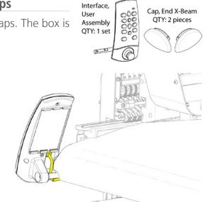
Route the network cable (shown in yellow) from under the right side machine cover, under the user interface mounting bolt, and plug into the back of the user interface assembly.
