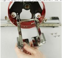
5. Assemble the 4 nuts onto the threaded posts by hand. Allow them to stay slightly loose. This will enable the adjustment of the support wing assembly to the machine.
