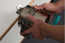
2. Unlatch the cap frame and swing the frame open and to the right.
