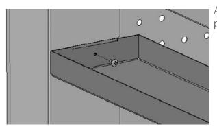
Align the holes in the tray and the cart legs. Tighten it into place using the two sheet metal screws (Items 2).
