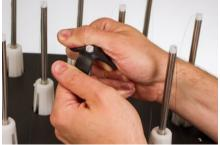
2. Collapse the clover to the thread tube as the cone is loaded onto the machine.
