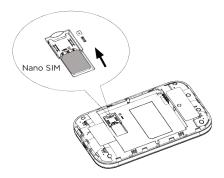
3. Insert the Nano SIM card. Install the battery and replace the back cover. When replacing the back cover, please ensure the back cover is aligned correctly.
