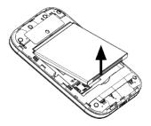
2. Remove the battery. Flip the device upside down and lift the battery upward gently as shown.
