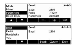
The current Baud Rate, Parity and Handshake settings are displayed on the screen.
