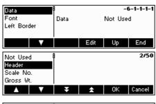
Choose "Date" to define the desired information for the line that was chosen. A detailed list of all functions can be found on the menu diagram (see Chapter 5.3.4 "COMMUNICATION  $\rightarrow$  Def. Heading Line  $\rightarrow$  Template 1-5  $\rightarrow$  Edit  $\rightarrow$  Line 1-23  $\rightarrow$  Data").
