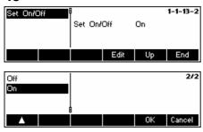
Press «Edit» to switch the minimum weight monitoring on/off.
