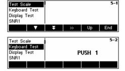
In order to check if all the keys are functioning properly, press **Yes** to start the keyboard test.
