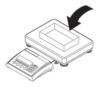
Place the **empty** weighing container or packaging on the platter and then press the **\*** T **\*** key briefly, or press the **\*** PT \* softkey if a **known tare weight** has already been established.
