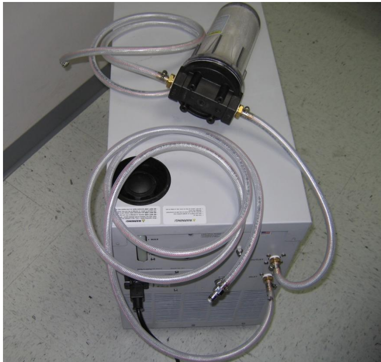
Figure 12. Picture of assembled water hoses, filter with the chiller
