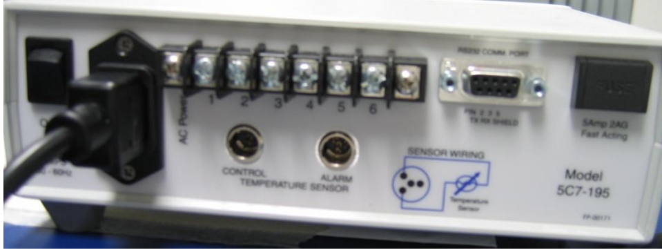
Figure 15. Picture of the back panel of TEC Controller
