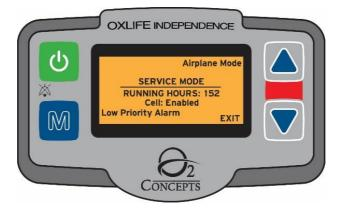
The unit will automatically enter the Low Priority Alarm test once the Medium Priority Alarm sequence has concluded. Pressing the Mode Button () while the Medium Priority Alarm test is in progress will terminate the Medium Priority Alarm test and start the Low Priority Alarm. The Low Priority Alarm consists of 1 beep and a solid amber LCD screen.
