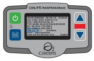
The voltage in is the voltage that the unit is receiving from an external power source, such as the AC power supply or DC power supply (ex. VIN: 23.7 where 23.7 is in volts).
